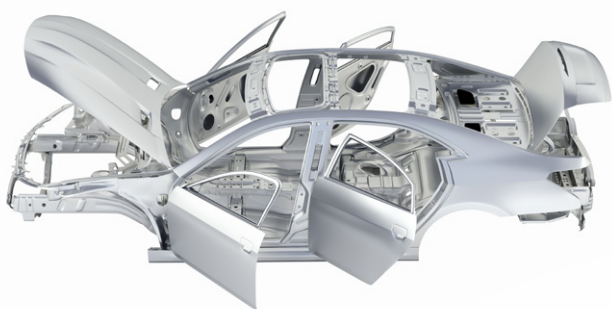
Figure 1. Car frames and body panels are often produced with advanced aluminum alloys.
